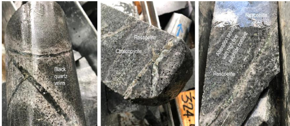
Figure 5: Hydrothermal breccia encountered between 422.5m - 426.5m in diamond drill hole TUDDH493. Monzonite fragments are intensely potassically altered. Cement is comprised of quartz-adularia-pyrite. Small pits called vugs are evident, some containing small particles of gold.
