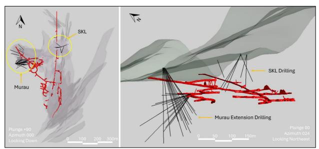
**Figure 1. Location of Murau extension and SKL near-mine expansion drillholes.** Left image: Plan view of Tuvatu showing Murau and SKL drillholes in relation to the mineralized lodes at Tuvatu, shown in grey. Right image: Oblique view of Murau and SKL drilling looking approximately northeast.
