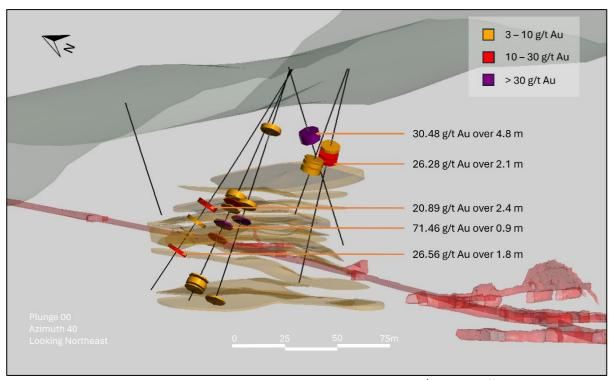
**Figure 3. SKL exploration drilling with high-grade intersects highlighted, 3.0 g/t gold cutoff.** The SKL lode system has historically been modelled as a series of stacked flat-lying mineralized lodes (light brown). The drillholes reported here are the first modern drillholes designed to target the SKL lodes and represent near-mine expansion of the Tuvatu resource. View is to the northeast.
