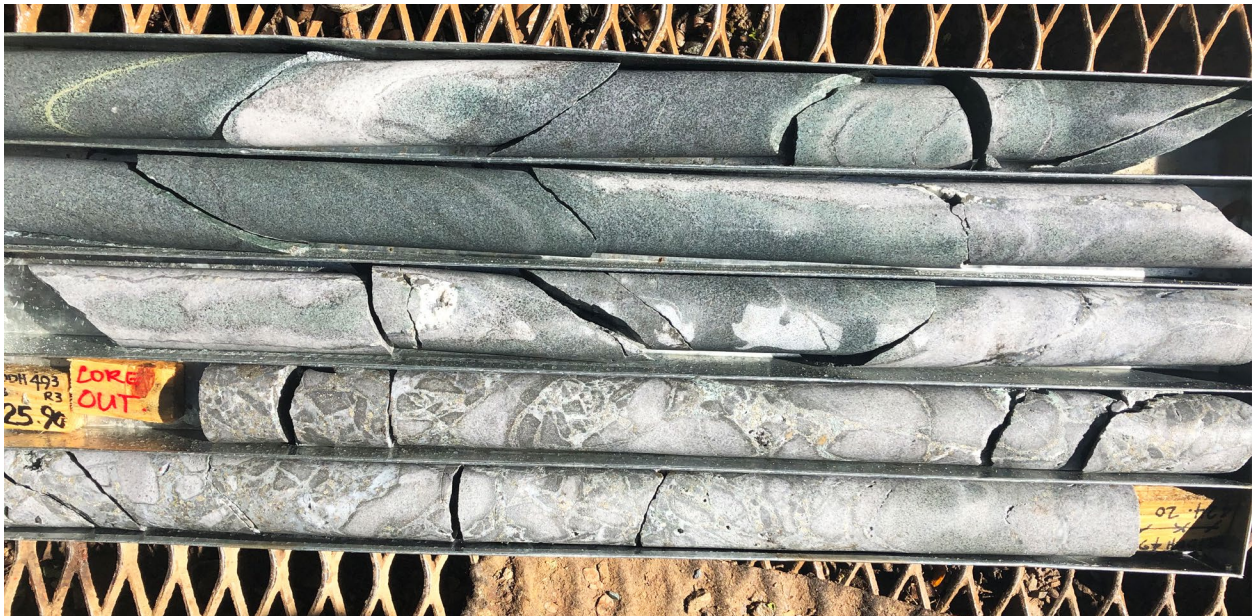
(Figure 2: Hydrothermal breccia encountered between 422.5-426.5 m in diamond drill hole TUDDH493. Monzonite fragments are intensely potassically altered. Cement is comprised of quartz-adularia-pyrite. Small pits called vugs are evident, some containing small particles of gold.)
