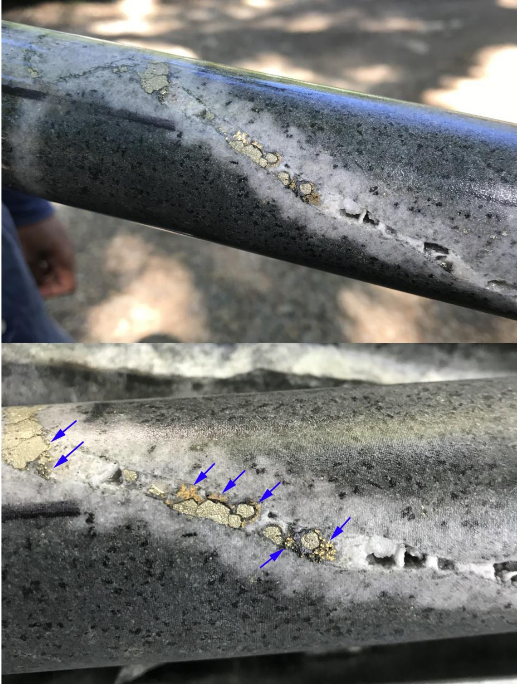
(Figure 1: Core from approximately 583 m down hole depth in hole TUDDH500. Photos show an approximately 1 cm wide quartz-adularia vein displaying coarse clots of visible gold, bright yellow, as well as pyrite, brassy yellow and galena and sphalerite, grey. Host rock is monzonite. Potassium feldspar flooding extends for up to 2 cm beyond the vein. Open space vugs are also present. Hole TUDDH500 has intersected notable veining beginning at a depth of approximately 570 m and is currently in progress toward its targeted depth of 1,000 m. The hole undercuts the entire Tuvatu lode system in an area where a root feeder is hypothesized to be located.) The photo is of a selected interval that is not necessarily representative of the mineralization hosted on the property.
