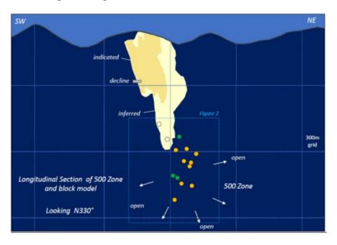
Figure 3: Longitudinal Section of Zone 500 and Block Model
