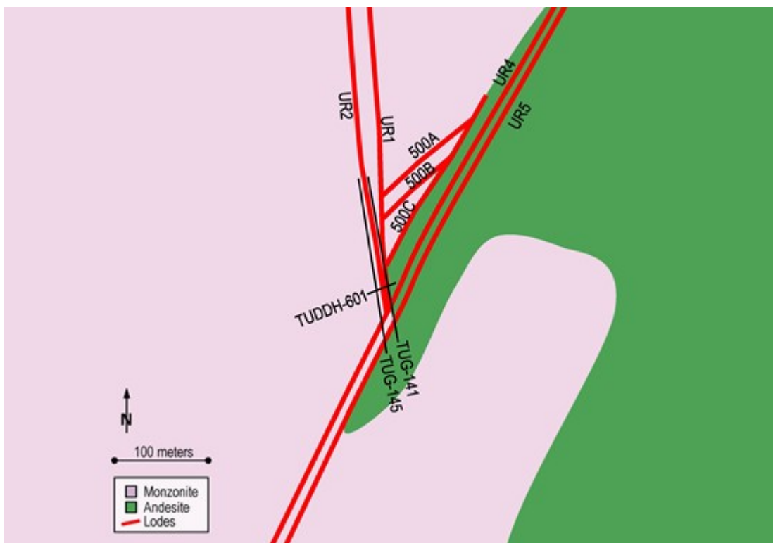
Figure 4. Schematic diagram of a horizontal plan at approximately RL= -260m illustrating the interpreted interplay between mineralized lodes and lithologic contact between monzonite (pink) and andesite (green), in the area of the TUG-141 high-grade discovery. The NE-trending monzonite-andesite contact is shifted to the south along UR1 at the location of the mineralization intersected by drill holes TUG-141 and TUDDH-601. Lodes UR1-UR2 pair appears to merge together at depth, with the NS-oriented lodes intersected by the NE-SW UR4 lode.
