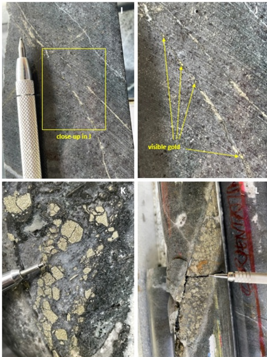
Figure 2 contd. I) TUDDH-601 at 592.2m showing very fine py-VG veins in pervasively altered andesite grading 33.77 g/t Au; J) close-up of photo I; K) TUDDH-601 at 609.0m qtz-py-roscoelite vein grading 10.49 g/t Au; L) TUDDH-601 at 610.8m qtz-py vein grading 20.31 g/t Au.
