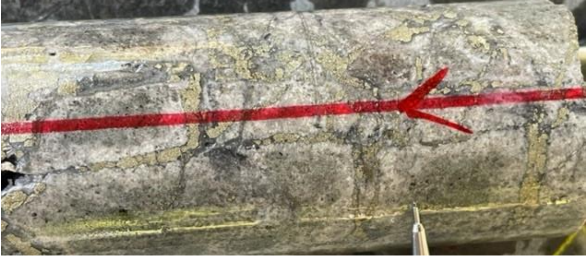
Figure 9: TUDDH 608. High-grade material hosted within mm-scale ladder vein at 606.5m. Grade: 54.54 g/t Au
