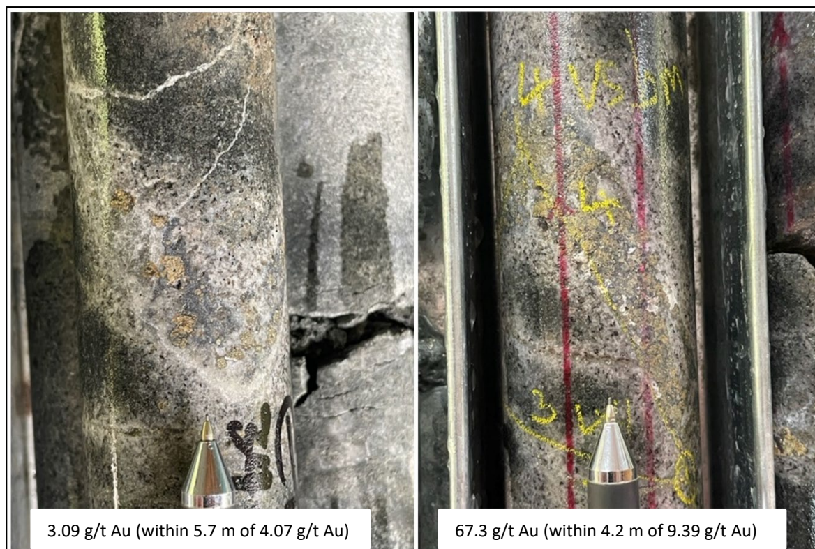
Figure 7. Examples of Zone 5 Drill Core. LEFT: UR2 lode in TGC-0049 at 35.15 m depth. Coarse grained honey sphalerite and pyrite in variable light to dark grey quartz vein with narrow potassic alteration halo. RIGHT: URW3 lode in TGC-0050 at 29.6 m depth. Abundant coarse honey sphalerite rimmed by fine grained sooty pyrite +/- galena and narrow potassic alteration halo, within a larger zone of stockwork style mineralization. Width of core is 4.76 cm in each photo.
