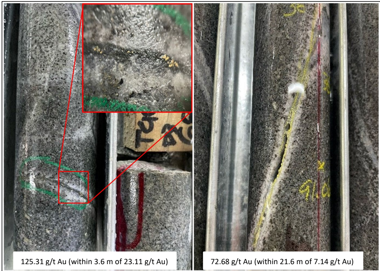
Figure 4. Example URW1 Drill Core. LEFT: TGC-0040 at 67.3 m depth. Monzonite-hosted stockwork-style veining with a narrow high-grade silica vein containing coarse grained visible gold. RIGHT: TGC-0042 at 91.60 m depth. Vuggy silica vein with narrow bleached alteration halo in monzonite. Width of core is 4.76 cm in each photo.
