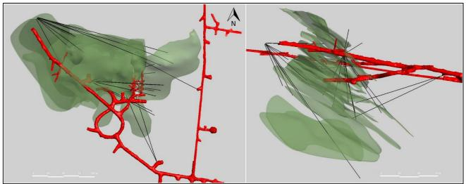
**Figure 3. Murau Lode System.** Plan view (left) and view looking east (right) of the Murau lode system in relation to the grade control drillholes reported here. Mining on the upper part of the Murau lode system is scheduled to start in Q4 2023. The stacked nature of the Murau lodes and their moderate dip to the south is visible in the right-hand image.
