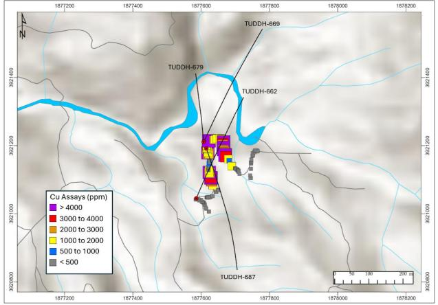
**Figure 3. Plan View of Wailoaloa Drillholes in Relation to Surface Sampling Results.** Bench sampling in the Wailoaloa area from 2019 to 2023 revealed a strong surface copper anomaly approximately 150 m x 100 m in size.
