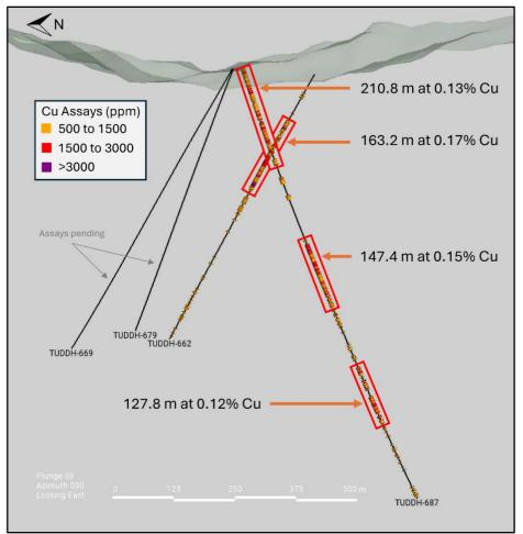
**Figure 2. Cross-Section of the Wailoaloa Drillholes, Looking East.** Zones of elevated copper mineralization are shown in red boxes. Three zones of anomalous copper mineralization are observed in TUDDH-687, and one in TUDDH-662. TUDDH-662 and TUDDH-687 both terminated in anomalous copper mineralization. Assays are pending for drillholes TUDDH-669 and TUDDH-679.
