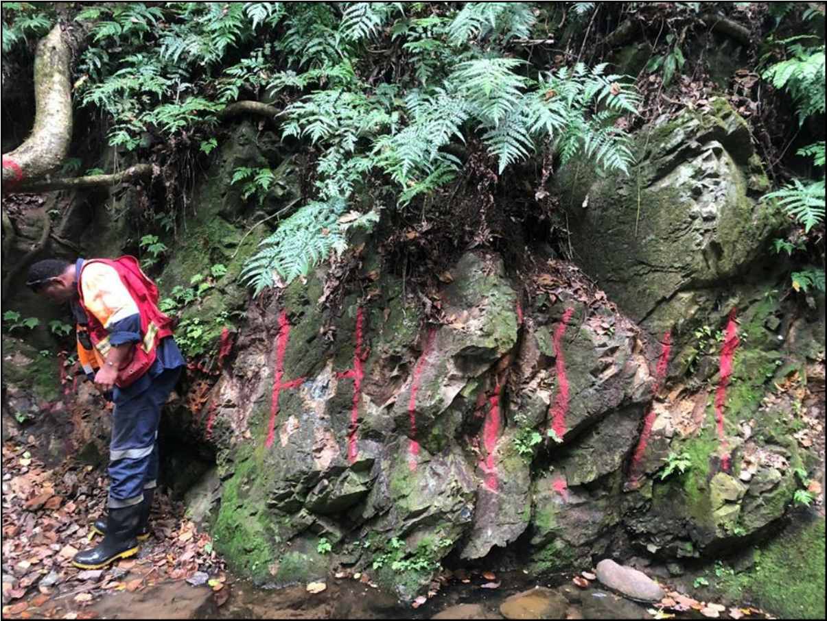
Figure 9.11 Channel Sample on an Outcrop with Paint Marks for Mapping and dGPS Surveying
