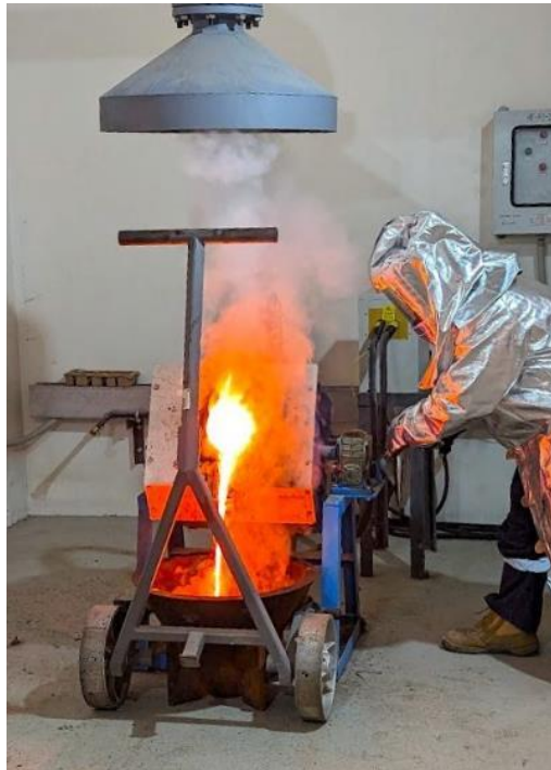
Figure 17.9 Doré Gold Pour with Electric Furnace
