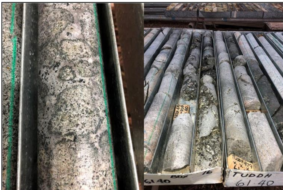
Figure 8.6 K-Feldspar + Silica Breccia Fill (left) (Alkalic Style) and High-temperature Secondary Biotite (Right) (Early Basemetal Style)
