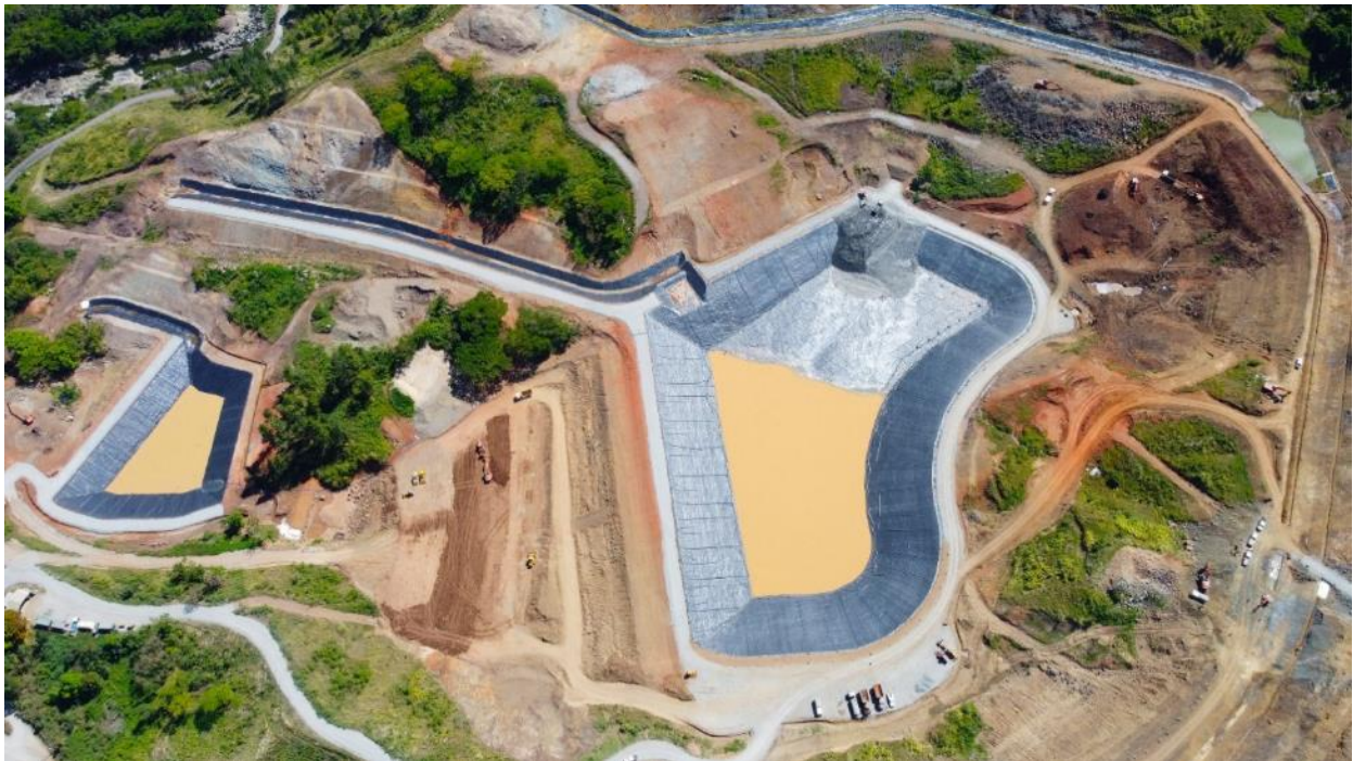
Figure 17.15 Aerial Photograph of Filtered Tailings placed in the TSF Pond to Build Ramp
