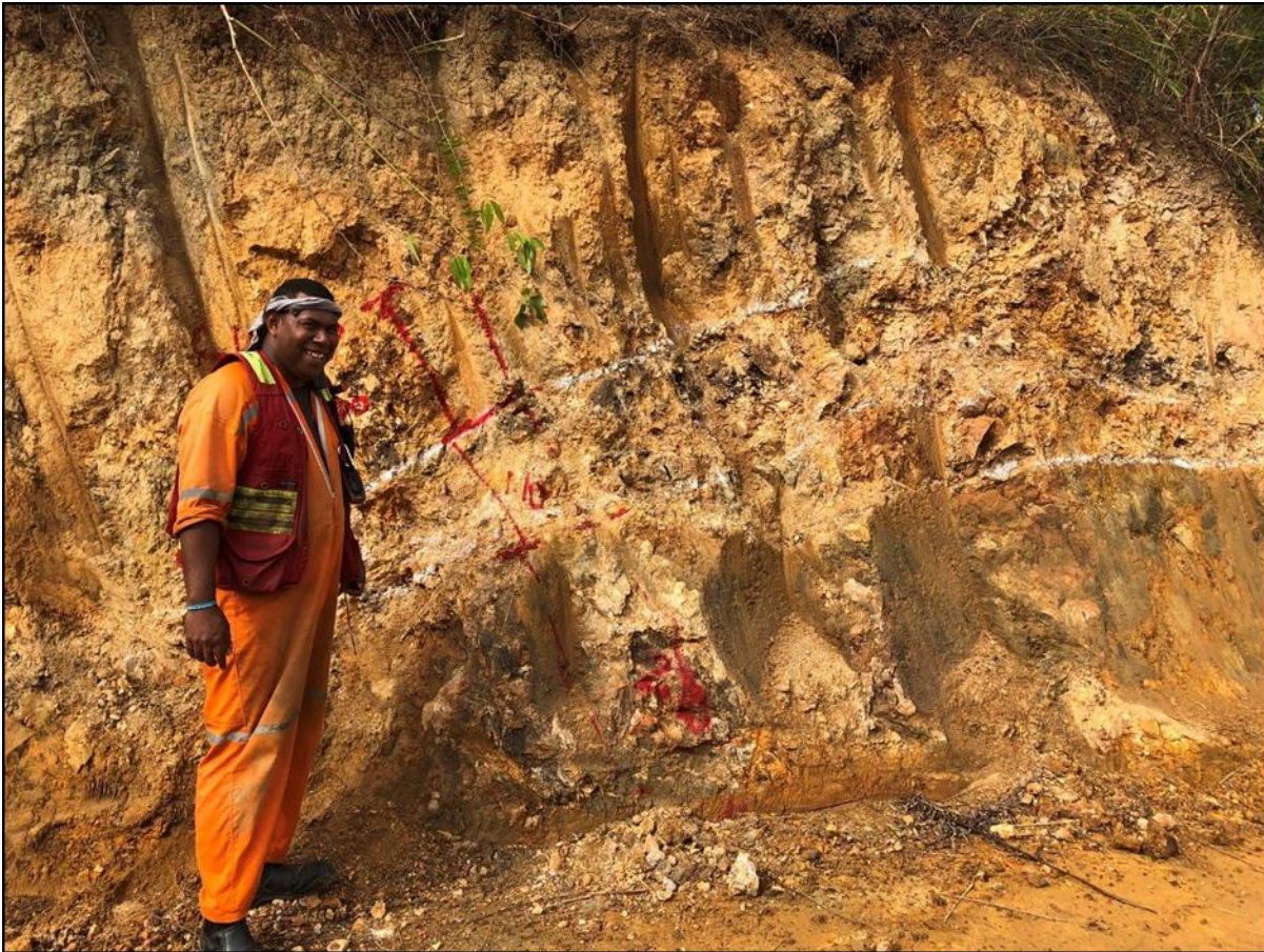
Figure 9.10 Example of a Channel Sample on a Bench with Paint Marks for Mapping and dGPS Surveying
