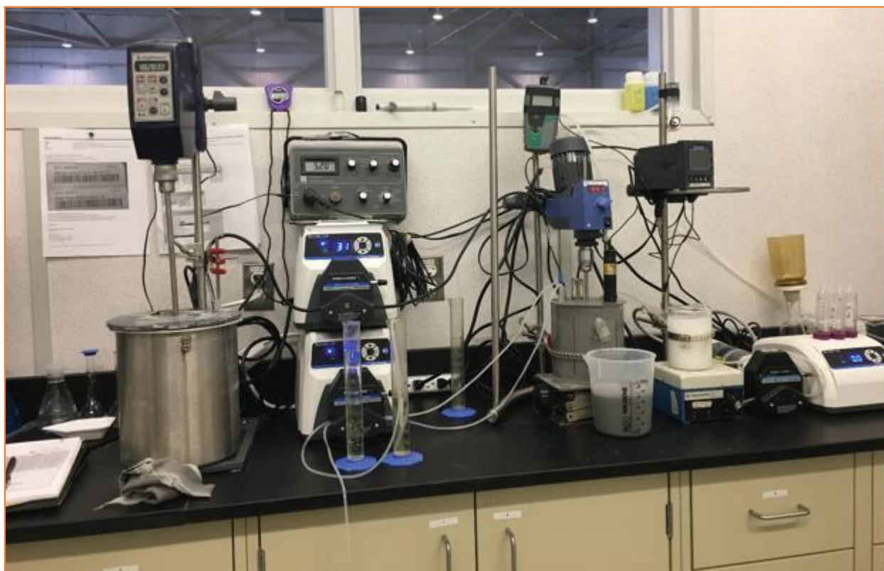
Figure 13.15. Kemetco Cyanide Test Setup
