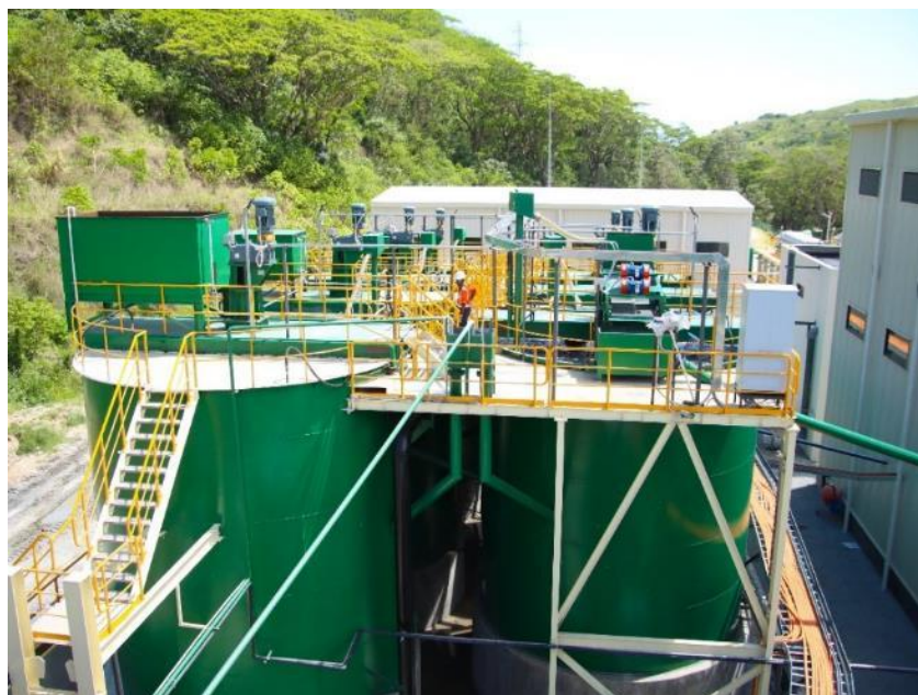
Figure 17.6 Pre-treatment tank (foreground) and six CIL tanks
