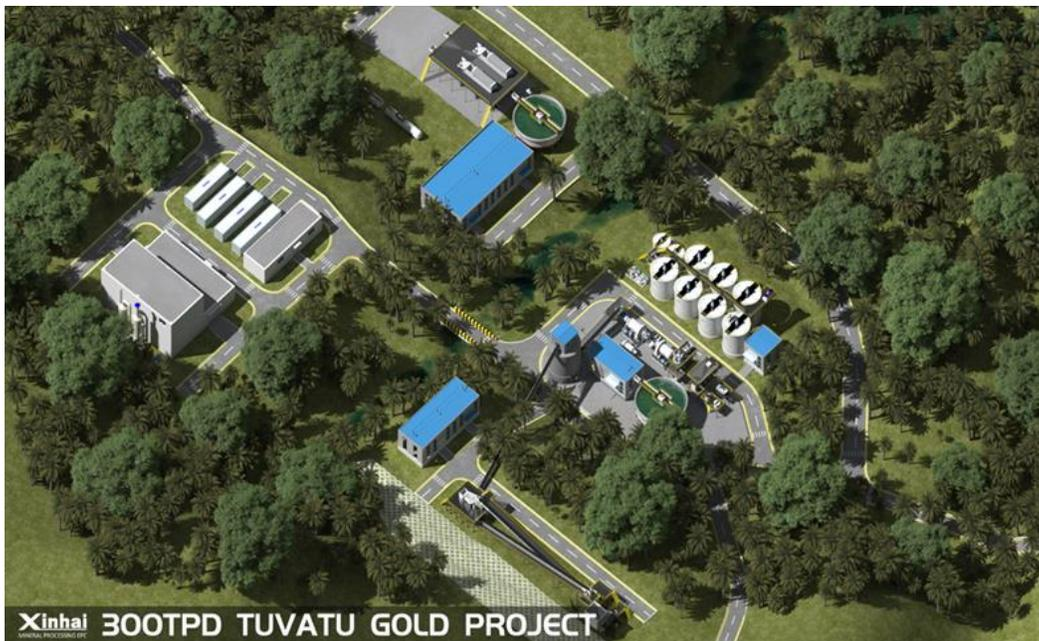
Figure 1: conceptual process plant design and site layout
