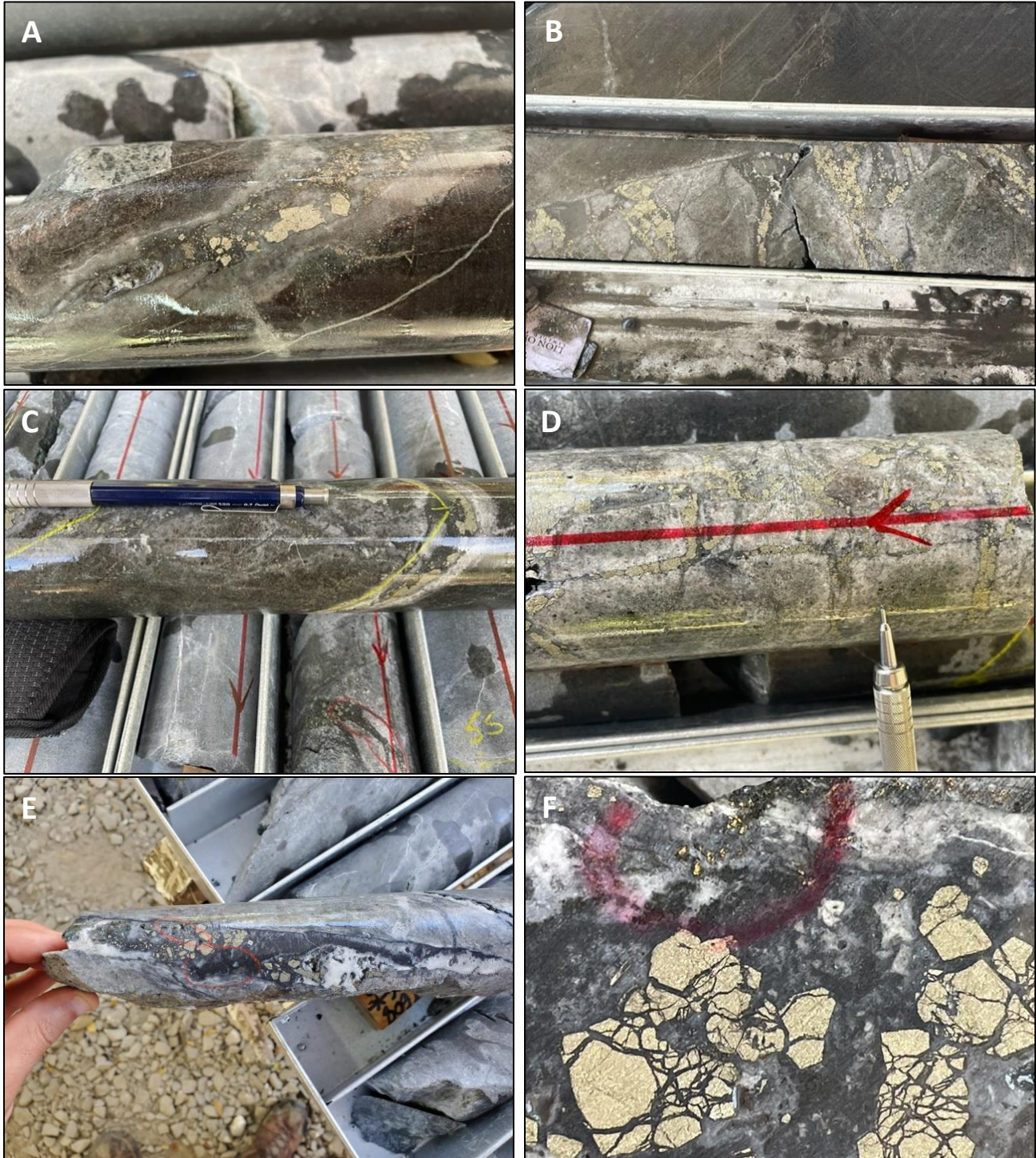
Figures 2: Photos from TUDDH-608 drill core, as follows: A) 571.5m, 17.03 g/t Au; B) 601.9m, 23.21 g/t Au; C) 599.5m, 108.31 g/t Au; D) 606.5m, 54.54 g/t Au; E) 611.8m, 45.02 g/t Au; F) close-up of cut core from photo E showing VG.
